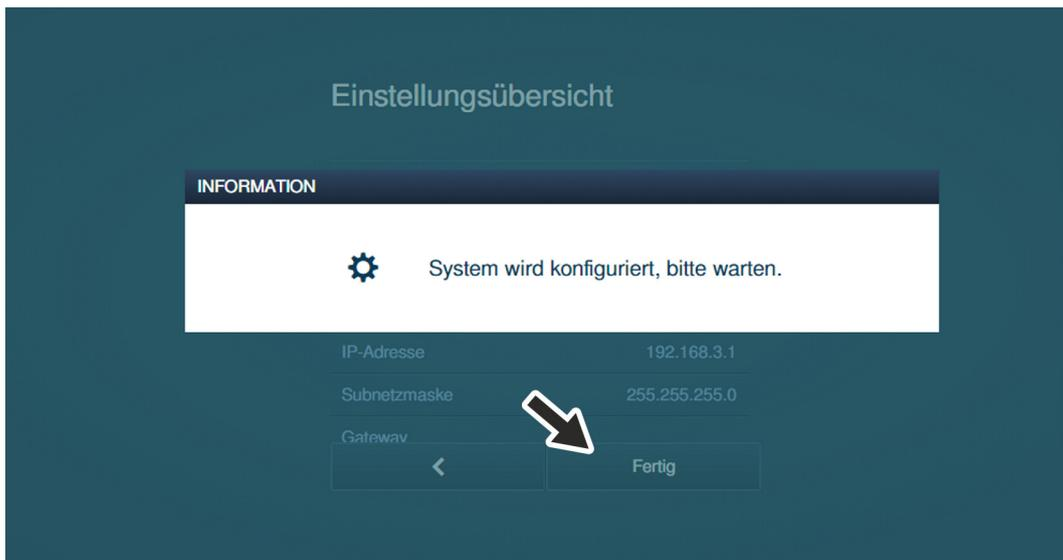
Fig . 79: Commissioning "Smart Access Point": Confirm settings
