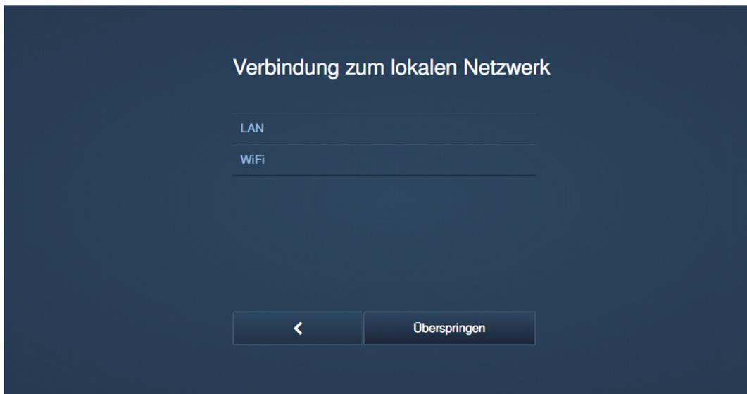
Fig. 70: Commissioning "Smart Access Point": Connection to the local network
