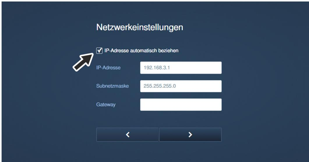
Fig. 71: Commissioning "Smart Access Point": LAN Network settings
