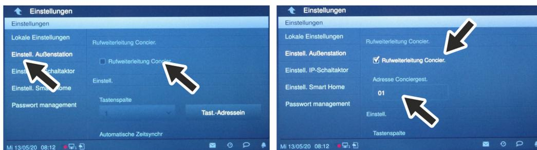
Fig. 55: Outdoor station with buttons: Setting the concierge call via the indoor station
